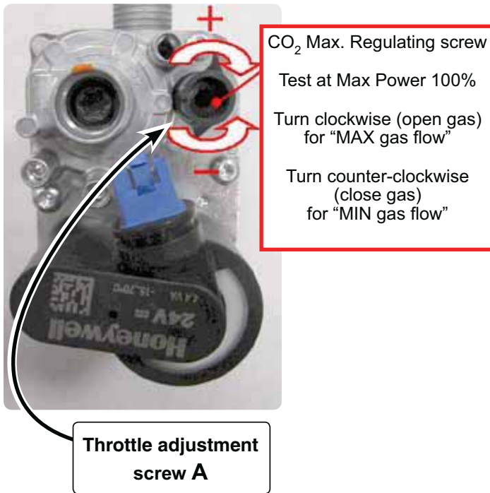
Figure 83 Throttle adjustment screw — (ONLY for use by a qualified technician, using calibrated combustion test instruments).
