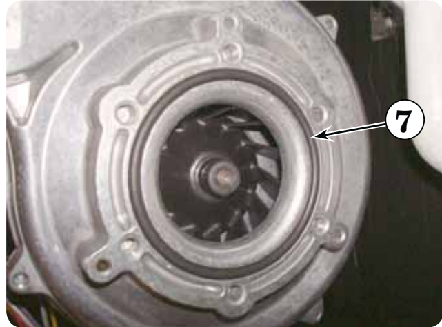
Figure 15 Insure "O" ring is in place
