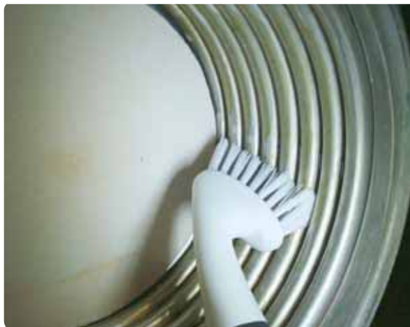
Figure 116 Cleaning the heat exchanger
