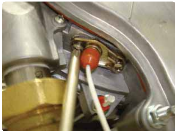
Figure 107 Removal of Ignition electrode
